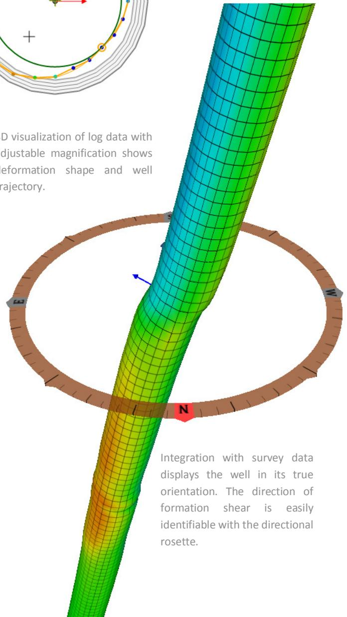
Integration with survey data displays the well in its true orientation. The direction of formation shear is easily identifiable with the directional rosette.
