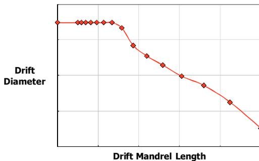
Calculate drift diameter dependence on mandrel length to evaluate well accessibility.
