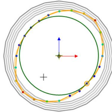
2D cross-section views show the extent of ovalization and clearance circle in deformed intervals..
